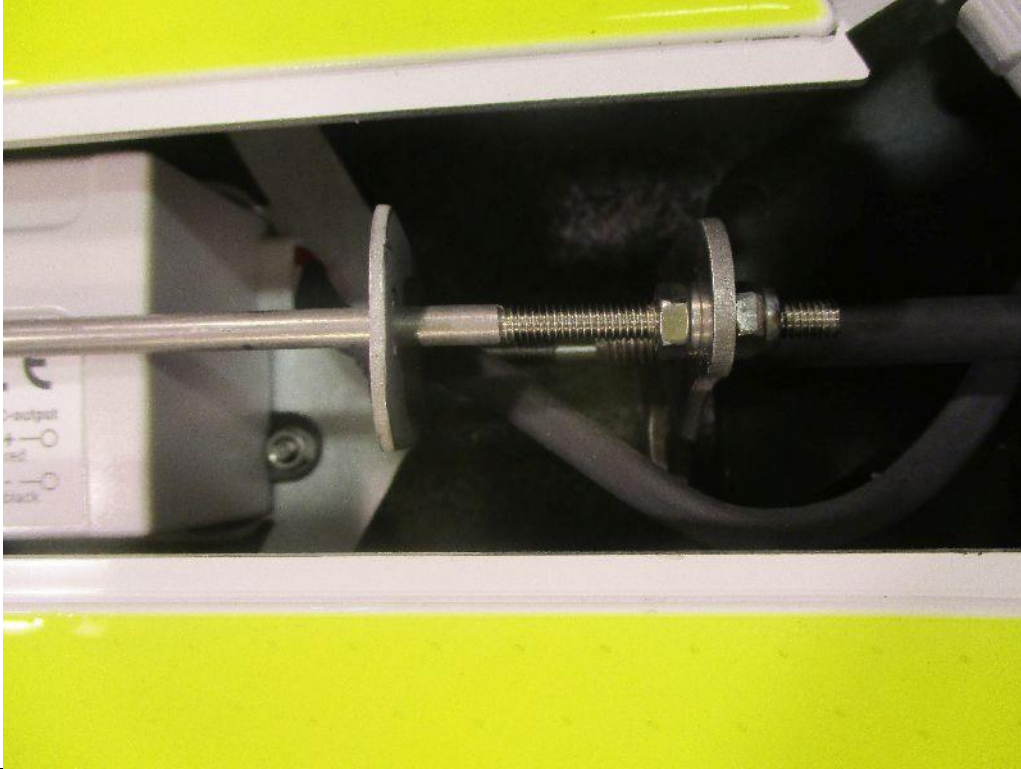
Bild / Picture 8: Securing of LED converter
